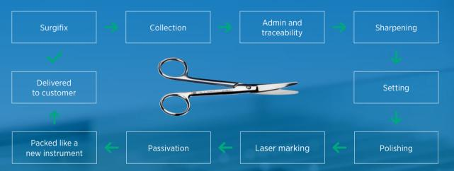
Every part of this process is important in order to repair the instrument to **'as new' condition**
